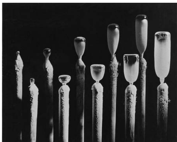
Fig. 16. Collection of ruby and sapphire crystals at different growth stages obtained by the verneuil method. Length of the longest crystal: ca. 12 cm (photograph by courtesy of DJÉVA-HIRDJIAN SA, CH-Monthey).
